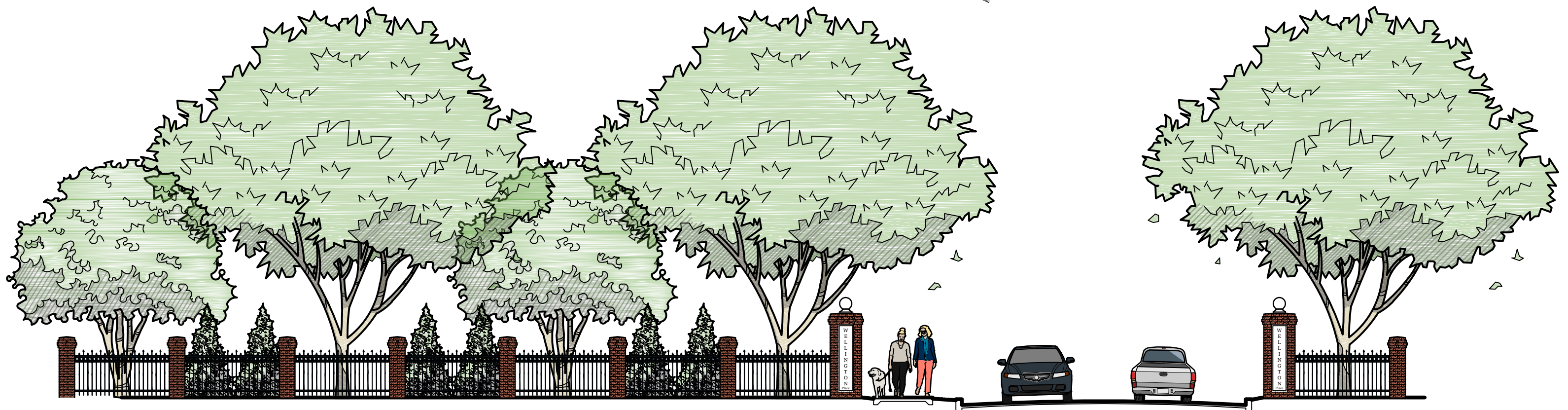
1 4' DECORATIVE FENCE WITH BRICK COLUMNS ELEVATION 1/8" = 1'-0"
